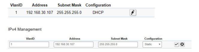
**Important--**If the device fails to retrieve an IP address through DHCP, the default IP address is 192.168.1.251 and the factory default subnet mask is 255.255.255.0.
