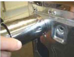
Figure 5. Screw the leg up tight so the oven base is clamped between the washer and the top of the leg. Once all four legs have been fitted lift cooker onto the legs taking care to distribute the weight evenly onto all four legs at the same time.
