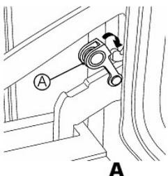
Open the oven door completely, insert the anti-rotation device (A) in the hook of the hinge rods. Hold the oven door by the sides and slowly close it until you can feel a certain resistance; simultaneously lift the door and force it towards its closed position in order to slide it out by freeing the hinge lock from the kitchen's body. To refit the door repeat the above instructions in reverse making sure the hinge lock is correctly fitted.
