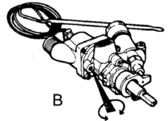
Adjust the previously loosened screws until the flame is lowered but stable, even when rapid changes are made from the maximum to the minimum position with the burner cold. If safety taps are fitted, let the burner run on minimum for a few minutes to ensure that the device does not cut in. If it does, increase the minimum.
