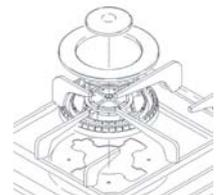
*Fish kettle:* fit the flame diffuser by placing the hole in the bottom part over the electronic ignition candle in the hob cup.
