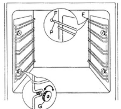
placing the 2 P extensions of the side guides in the holes F on the bottom of the oven; line up the 2 front eyelets of the guides with the screws fitted to the sides, then secure the guides with nuts/washers G. Do not wash the oven when it is still hot and do not use abrasive substances or products.
