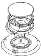
*Treble crown burner:* fit the flame diffuser to the burner support so that it cannot rotate.
