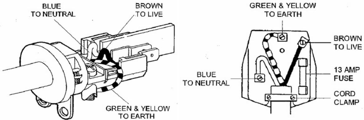
The wired in the mains lead are coloured in accordance with the following code:
