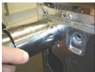
Figure5. Screw the leg up tight so the oven base is clamped between the washer and the top of the leg. Once all four legs have been fitted lift cooker onto the legs taking care to distribute the weight evenly onto all four legs at the same time.
