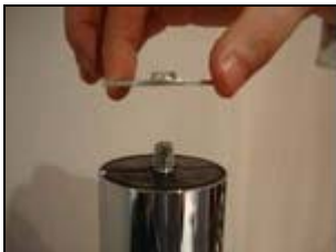
Figure1. When fitting the washer to the leg bolt make sure the burr on the washer is facing upward away from the leg top.
