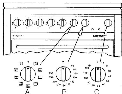
between 50 and 250°C; therefore even the most varied cooking requirements are satisfied. Depending on the models, these cookers have an end of cooking timer or a digital electronic programmer.
