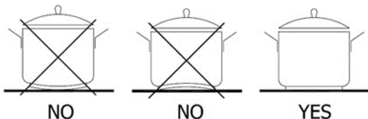
Each cooking zone is equipped with a "pan present" device, which ensures that cooking cannot start unless a suitable pan is placed on the cooking zone and properly positioned.
