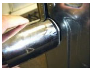
Figure 4. Insert washer fitted to top of leg into base of cooker and slide the leg along the channel.
