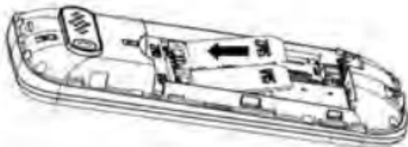
2. Take out SIM card: Hold the notch of SIM card and lift it slightly down by the other hand to take card out.
