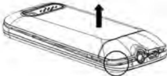
2. Put battery into the battery slot. Keep three metal points of battery facing downward and matching with the three
