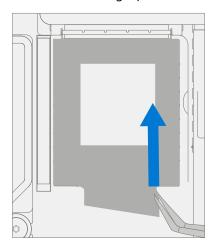
2. **Remove rSSD screw** – Using a 5IP (Torx-plus) driver remove the screw securing the rSSD.
