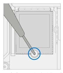
3. **Apply desense** – On the **15" model only**, there is a desense sticker covering the rSSD. Carefully align the desense sticker over the rSSD and apply.
