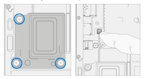
2. **Install right speaker** – Place right speaker in chassis. Using a 3IP (Torx-plus) driver install the 3 screws securing the right speaker to the chassis until finger tight. Then turn each screw an additional ~45-degrees (1/8 turn), or until fully fastened. Connect speaker to motherboard.
