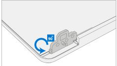
2. **Install display module onto chassis** – While holding the display with one hand. Carefully align the hinges into the pockets on the chassis.
