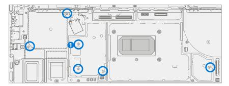
3. **Install stiffening bar** – Using a 3IP (Torx-plus) driver install the 2 stiffening bar screws securing the stiffening bar to the motherboard and chassis.
