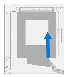
7. **Remove rSSD screw** – Using a 5IP (Torx-plus) driver remove the screw securing the rSSD. Take care not to damage the screw; it will be reused.
