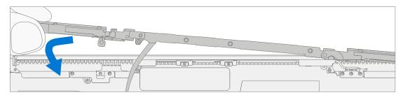
5. **Install WiFi clip** – Using a pair of tweezers, align WiFi clip with screw holes. Then use a 3IP (Torx-plus) driver install 2 WiFi clip 2 screws until finger tight. Then turn screw an additional ~45-degrees (1/8 turn), or until fully fastened.
