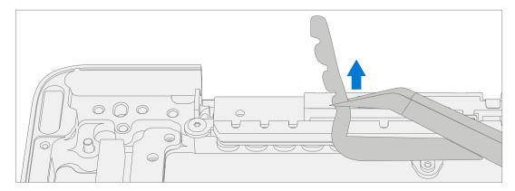
3. **Remove WiFi deck screws** – Using a 3IP (Torx-plus) driver remove the 12 screws that hold in the WiFi deck.
