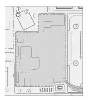
4. **Remove stiffener bar** – On right side of motherboard, using a 3IP (Torx-plus) driver remove the 2 screws securing the stiffening bar to the motherboard and chassis.
