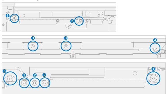
7. Install rubber caps – Install rubber caps on chassis standoff where shown below.
