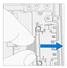
2. **Connect Surflink FPCs** – Align the FPC's connectors to the motherboard and slide into connector. Press down on locking cover.
