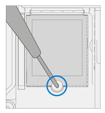
12. **Apply desense** – On the **15" model only**, there is a desense sticker covering the rSSD. Carefully align the desense sticker over the rSSD and apply.
