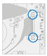
4. **Install bracket** – Place the Surflink bracket over the Surflink. Using a 3IP (Torx-plus) driver install 4 new Bracket Screws. Turn all screws until they are just snug and seated, and then turn another 45-degrees (1/8 turn) or until fully fastened.
