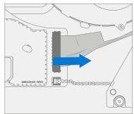
3. **Remove Surflink Port Screws** – Using a 3IP (Torx-plus) driver remove the 2 Surflink Screws securing the Surflink Port to the chassis.
