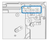
4. **Pre-fasten left hinge screws** – Using a 6IP (Torx-plus) driver assemble 3 new Hinge Screws in the left-side hinge and tighten until just snug.
