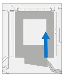
4. **Apply TIM** – Apply a thermal pad to the rSSD approximately as shown in image below.
