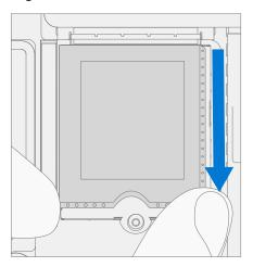
2. **Install new rSSD screw** – Using a 5IP (Torx-plus) driver install the rSSD screw. Turn the screw until just snug and seated, and then turn another 45 degrees (1/8 turn) or until fully fastened.
