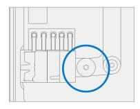
4. **Position WiFi deck** – Align the WiFi deck to the posts on the Chassis. Be sure to make sure the black WiFi antenna is not pinched between the chassis and the deck.
