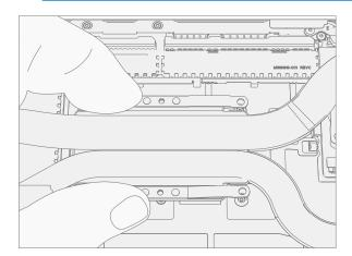
2. **Install socket screws** – Using a 3IP (Torx-plus) driver install the 4 new socket screws in each corner tensioner. Turn each screw until just snug and seated, and then turn another 45 degrees (1/8 turn) or until screws are fully fastened.
