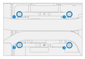
5. **Remove thermal module** – Using a plastic spudger gently work under the edge of the thermal module to break the seal with the TIM underneath. Lift out thermal module.
