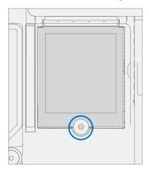
3. **Remove rSSD** – The rSSD should lift upwards to ~15-degrees after screw is removed. Carefully grab sides of rSSD case and pull out of main board socket at same ~15-degree angle.
