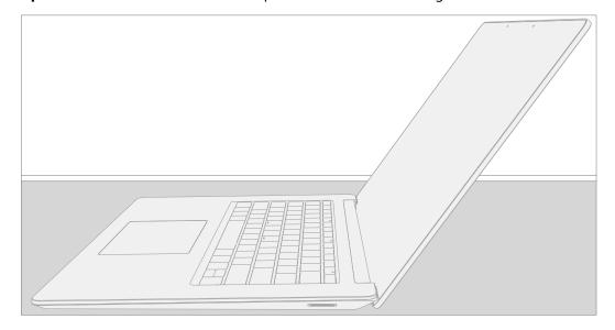
3. **Separate keyboard from device** – Grasp the back of the keyboard, by the display, and pull directly up. Keyboard should lift free from the device.
