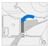
3. **Install new Surflink Screws** – Using a 3IP (Torx-plus) driver install 2 new Surflink Screws. Turn all screws until just snug and seated, and then turn another 45-degrees (1/8 turn) or until fully fastened.
