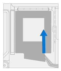
13. **Apply TIM** – Apply a thermal pad to the rSSD approximately as shown in image below.
