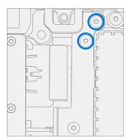
4. **Install right shield** – Align shield with shield retainer. Press along the edge of the shield until the shield is fully seated.
