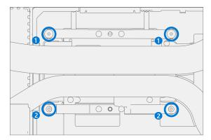
3. **Install thermal module screws** – Using a 3IP (Torx-plus) driver install the 5 new Thermal Module Screws that secure it to the chassis. Turn each screw until just snug and seated, and then turn another 45-degrees (1/8 turn) or until screws are fully fastened.
