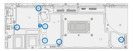
6. **Remove motherboard** – Grab the right-hand side of the motherboard and lift until just of the chassis standoffs while gently rotating it toward you and pulling gently to the right. A wiggling motion will be required to loosen the top of the board from the chassis. Lift the motherboard out of the Chassis.
