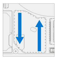
5. **Install left shield** – Align shield with shield retainer. Press along the edge of the shield until the shield is fully seated.
