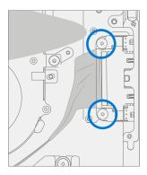
4. **Remove Surflink Port** – Remove the Surflink Port from the chassis.
