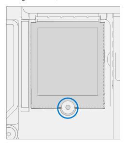
8. **Remove rSSD** – The rSSD should lift upwards to ~15-degrees after screw is removed. Carefully grab sides of rSSD case and pull out of main board socket at same ~15-degree angle.
