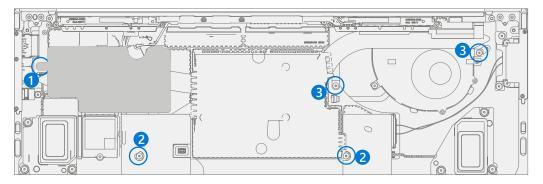
**IMPORTANT:** The 15" model has six screws on the thermal module. Locations are listed below.
