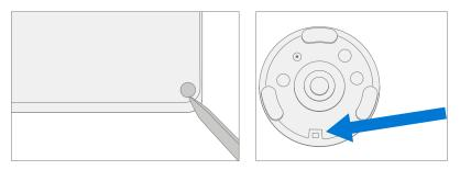
2. **Remove back feet** – Use a plastic tool to pry up the back foot from back divot and then peel to remove. Repeat for the other foot.
