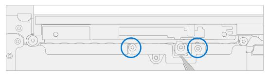
6. **Install WiFi deck screws** – Using a 3IP (Torx-plus) driver install the 10 marked WiFi deck screws until finger tight. Numbers correspond to the relevant WiFi deck screw. Then turn screw an additional ~45-degrees (1/8 turn), or until fully fastened.
