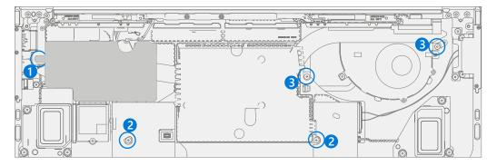
**IMPORTANT:** The 15" model has 6 screws on the thermal module. Locations are listed below.
