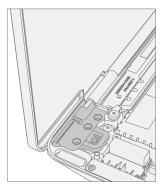
3. **Pre-fasten right hinge screws** – Using a 6IP (Torx-plus) driver assemble 3 new Hinge Screws in the right-side hinge and tighten until just snug.
