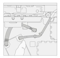
9. **Secure WiFi deck** – Using the screw retained in Procedure – Removal (Display) step 3 and a 3IP (Torx-plus) driver, tighten the WiFi deck back down onto the chassis until finger tight. Then turn the screw an additional ~45-degrees (1/8 turn), or until fully fastened.
