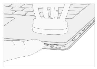
5. **Angle C-cover** – Angle the C-cover at approximately 45 degrees from horizonal – be sure to angle the keyboard **no more than 45 degrees** or else risk damaging the keyboard hook or FPC. If hook is damaged, it needs to be removed carefully to avoid damaging the FPCs, and then a new keyboard needs to be installed.
