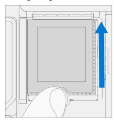
11. **Install rSSD screws in both devices** – Use a 5IP (Torx-plus) driver to install a new rSSD screw until the screw is just snug and seated, and then turn another 45-degrees (1/8 turn) or until screw is fully fastened.
