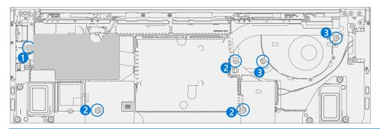
4. **Install thermal module shield** – Align shield around retention frame and press down the upper left corner. Then work around the outer edge of the shield, there should be clicking as the shield seats properly.
