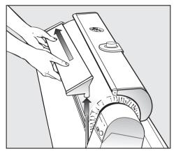
First remove the feed-in table by lifting it out of the right hand holder, and then pulling it out to the left of the roller. Then insert the plug in the socket and switch the ironer on. The heater plate will rise automatically.
