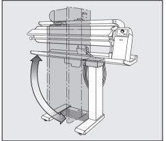
Swing the top section of the ironer to the horizontal position for using it, or swing it down in the vertical position for storage. Then let go of the release catch.
