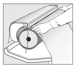
Insert the raw edge of the new ironing cloth into the retaining slot with the wrong side down. Leave the cords hanging free and smooth out the cloth.
