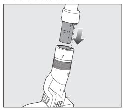
■ Push the suction tube connector into the electrobrush from above until it audibly clicks into place.
