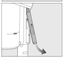
Clean the dust container and pre-filter with a dry cloth or with a cleaning tool which is located on the side of the PowerUnit.
