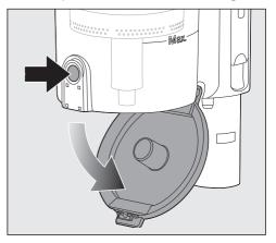
Press the release button on the bottom of the dust container.
