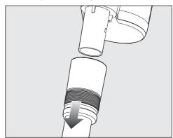
■ Slide the sliding ring on the suction tube down to separate the individual sections from each other.
