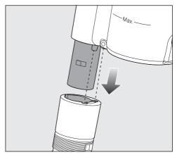
■ Push the PowerUnit connector into position in the suction tube until it audibly clicks into place.
