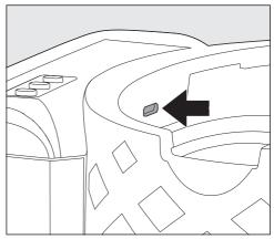
Use a flat-head screwdriver to carefully release the battery compartment cover.
