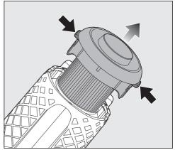
Remove the fine dust filter from the PowerUnit.
