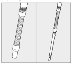
The hose extension can be extended to a maximum length of 120 cm. It can be extended further using the extendable flexible crevice nozzle.
