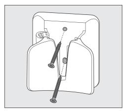
■ Attach the wall bracket to the wall.
