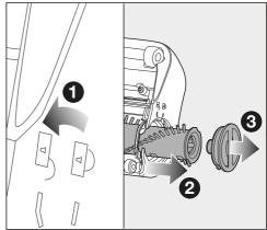
1 Turn the arrow on the handle on the side of the electrobrush to the ☐ symbol.
