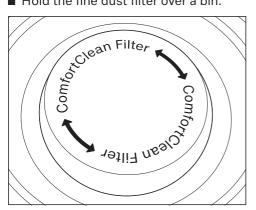
■ Take hold of the black section of the fine dust filter underneath the screw cap and turn the screw cap 10 times through 180°.
