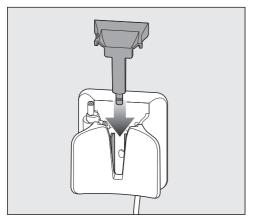
■ Slide the cover down into the wall bracket from above until it audibly clicks into place.
