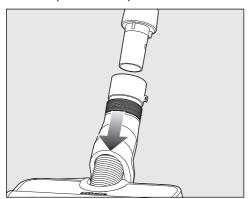
Slide the sliding ring on the electrobrush down to separate the individual sections from each other.
