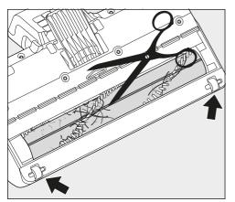
Cut any threads or hairs that have wound themselves around the roller brush with a pair of scissors. To guide the scissors, there are two guide tracks on the roller brush.
