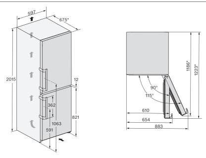
$<sup>^{\</sup>star}$  Dimensions without wall spacers fitted. Appliance depth is increased by 15 mm with the wall spacers supplied fitted.
