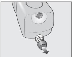
Remove the cover cap from the cartridge.
