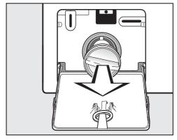
■ Remove the drain filter completely.
