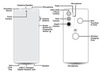
Use a digital headset: To use a digital headset, you'll need one with a USB-C connector. If using a 3.5mm digital headset, you'll need an adapter to connect a 3.5mm connector to USB-C. Digital headset may be sold separately.
