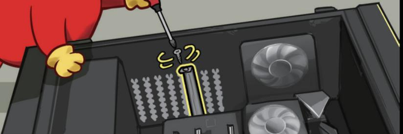
Make sure you release the small plastic latch on the end of the PCI-E slot on your motherboard to unlock your old graphics card. Now you can gently lift the old graphics card out of the case.
