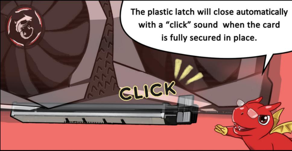
The plastic latch will close automatically with a “click” sound when the card is fully secured in place.
