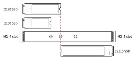
When installing a 2280 SSD in M2\_5 slot, a 2260, 2280, or 22110 SSD can be installed in M2\_4 slot.
