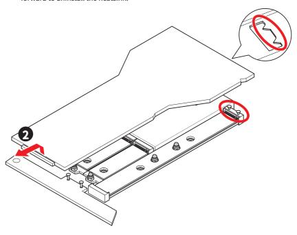
3. Remove the protective film from the M.2 thermal pads on the M.2 plate.
