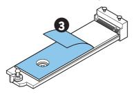
If you install 2260 SSD, use the included EZ M.2 Clip II Remover. Remove the plate screw and install EZ M.2 Clip II in the slot by using the remover. Skip this step if you install 2280 SSD.
