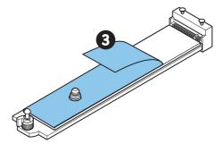
If you want to install 22110 SSD, use the included EZ M.2 Clip II Remover to remove the EZ M.2 Clip II in the 2280 hole. And then secure the included M.2 plate screw in the 2280 hole. Skip this step if you install 2280 SSD.
