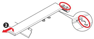
If you want to install the 2260 SSD, replace the EZ M.2 Clip II to the 2260 hole. Please note that you have to use the EZ M.2 Chip II Remover to remove and install the EZ M.2 Clip II. Skip this step if you install 2280 SSD.
