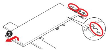
If you want to install the 2260 SSD, replace the EZ M.2 Clip II to the 2260 hole. Please note that you have to use the EZ M.2 Chip II Remover to remove and install the EZ M.2 Clip II. Skip this step if you install 2280 SSD.
