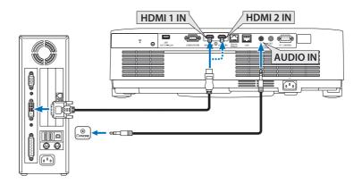
Connect the audio output of the computer to the projector's AUDIO IN terminal. In this case, switch the [HDMI1] or [HDMI2] setting at [SETUP]  $\rightarrow$  [OPTIONS(1)]  $\rightarrow$  [AUDIO SELECT] the on-screen menu to [COMPUTER]. ( $\rightarrow$  page 75)
