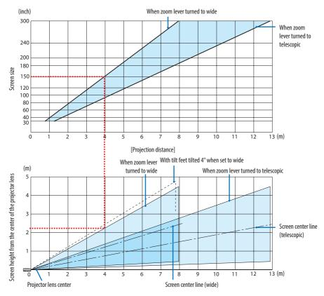
\* The figures indicated for "height of screen from projector lens center" on the projection distance table are for a lens shift of 60% V.
