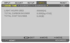
The [CARBON SAVINGS-SESSION] message shows the amount of CO<sub>2</sub> emission reduction between the time of changing to ECO MODE immediately after the time of power-on and the time of power-off. The [CARBON SAVINGS-SESSION] message will be displayed in the [POWER OFF / ARE YOU SURE ?] message at the time of power-off.
