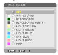
This function allows for quick adaptive color correction in applications where the screen material is not white.
