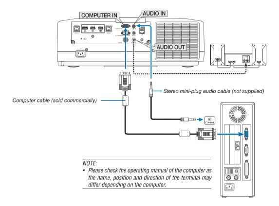
• Select the source name for its appropriate input connector after turning on the projector.
