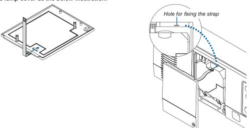
2. Insert the opposite side of the lamp cover strap to the hole on the projector body.
