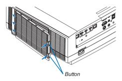
This completes the filter replacement. Go on to clear the filter hours.
