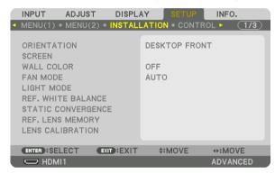
4. Press the ▼ button to select [REF. LENS MEMORY] and press the ENTER button.
