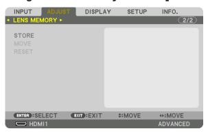
This function serves to store the adjusted values for each input signal when using the LENS SHIFT, ZOOM and FO-CUS buttons of the projector. Adjusted values can be applied to the signal you selected. This will eliminate the need to adjust lens shift, focus, and zoom at the time of source selection.
