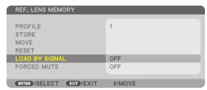
2. Press the ▼ button to select and [ON] and press the ENTER button.
