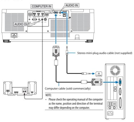
• Select the source name for its appropriate input connector after turning on the projector.
