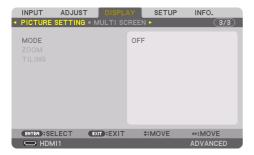
This sets the division conditions for reducing or enlarging the image area and displaying it in the desired position or for projecting using a combination of several projectors. Please refer to "4. Multi-Screen Projection" ( $\rightarrow$  page 66) for details.
