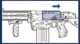
1. Pull SLIDE all the way back until READY INDICATOR is orange; keep in the rearmost position.
