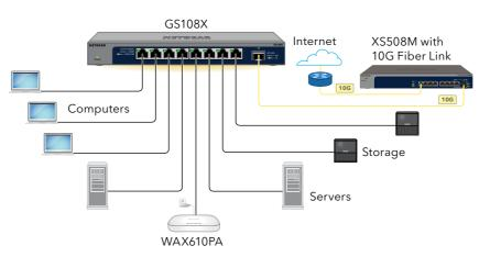
**NOTE:** We recommend that you use a Category 6a (Cat 6a) cable or higher roted cable for 10 Circle 15 Circ higher-rated cable for 10-Gigabit Ethernet connections, and a Category 5e (Cat 5e) cable or higher-rated cable for other Gigabit Ethernet connections.
