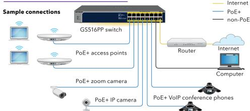
Note: This switch is designed for indoor use only. If you want to connect to a device located outdoors, the outdoor device must be properly grounded and surge protected, and you must install an Ethernet surge protector inline between the switch and the outdoor device. Failure to do so can damage the switch.
