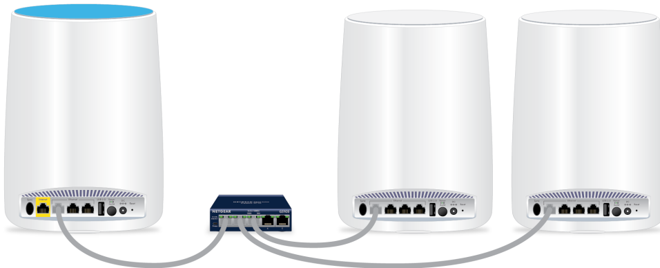
Figure 15. Ethernet backhaul connection using a switch
