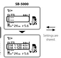
Flash function settings for remote flash units are changed on the SB-5000.
