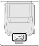
To use an external power source, remove the external power source terminal cover and connect the power cord to the terminal.
