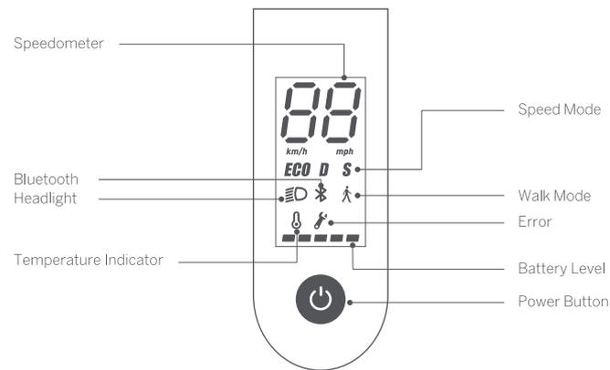
**Power Button:** Press the button to turn the KickScooter on; press and hold the button for 3 seconds to turn the KickScooter off. When the KickScooter is on, press the button to turn the headlight and rear light on/off; press twice to switch between speed modes.
