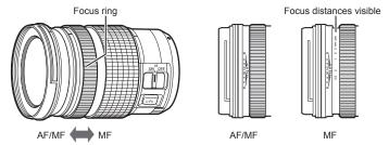
· Selecting [MF] for focus mode on the camera disables autofocus even when the focus ring is in the AF/MF position.
