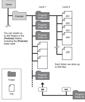
The recorder will not detect files in folders copied from a computer to the second level of folders.
