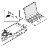
• [Remote] appears in the recorder display when the recorder is connected to a computer via USB.
