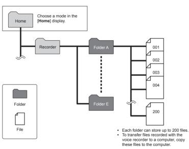
• Files and folders stored directly under the [Recorder] folder are not displayed on the voice recorder.
