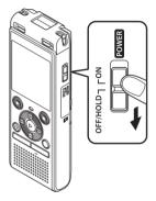
The playback stop position at power OFF is stored in the memory.
