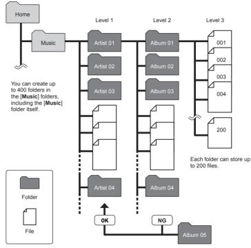
• The voice recorder cannot play files other than files in the MP3/PCM format transferred from a computer. The recorder will not detect files in folders copied from a computer to the second level of folders.
