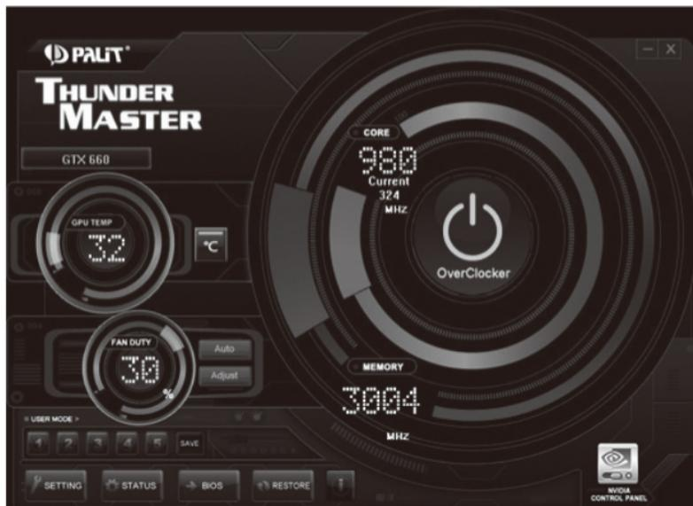
**ThunderMaster UI** shows the important information such as GPU clock speed, memory clock speed, fan duty cycle and GPU temperature. And, a lot more features to provide advanced user more detail information for over-clocking. The newer version is easier to understand and easier to use, everything you need is on one single well organized page!
