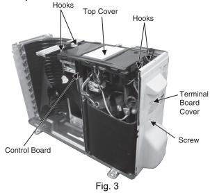
5 Remove the Control Board as follows:
