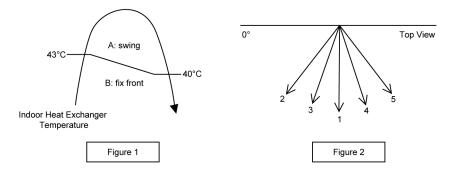
Manual horizontal airflow direction can be set using remote control; the angles of the vane are as stated below and the positions of the vane are as Figure 2 above.
