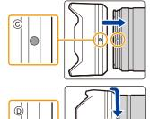
2 Rotate the lens hood in the direction of the arrow until it clicks and then align the mark ① ( ) on the lens hood with the mark on the tip of the lens.
