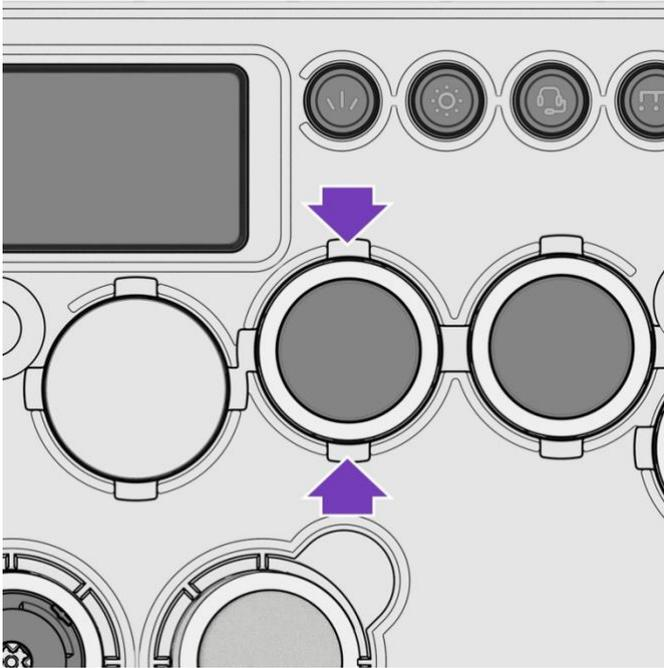
D. Remove the Button Cap with the Switch Puller
