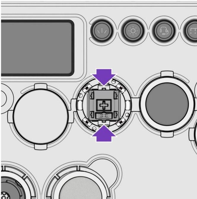
F. Place the Switch in the dedicated storage area, being mindful to avoid damaging the metal contact pins under the switch.
