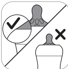
2. Make sure you pull the teat through until its lower part is aligned with the screw ring.
