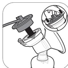
6. Attach the silicone tube and cap onto the silicone diaphragm. Push down the cap until it is securely in place.
