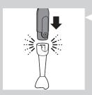
1 Attach the blender bar to the motor unit ("click").
