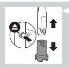
12 Remove the gear unit by pressing the release button.
