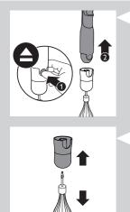
9 Press the release button to remove the motor unit from the gear unit.
