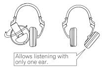
In order to support a wide variety of monitoring styles, this product has been designed with the ability to swivel the ear pieces front-to-back, and rotate each earpiece housing to the outside. Before using, however, please confirm the correct direction and degree of movement allowed, and do not apply excessive force in the attempt to swivel, rotate, or bend the headphones in ways not supported, since damage may result.
