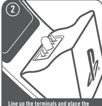
Line up the terminals and place the controller onto the charger
