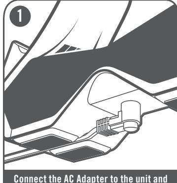
Connect the AC Adapter to the unit and plug into an electrical outlet
