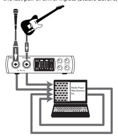
**Power User Tip:** When using either option, you will need to select Outputs 1 and 2 in the audio application your want to record. Make sure to select Outputs 3 and 4 in the audio application in which your recording to avoid a feedback loop.
