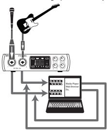
When Loopback is enabled and "Dedicated Loopback Inputs" is selected, the audio from another application will be recorded on the last pair of driver inputs (Studio 26: 5/6, Studio 68: 7/8).
