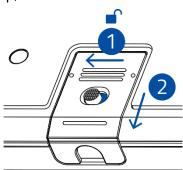
2. Lift the security clasp and connect the USB Type C to USB Type A cable to the USB Type C port of the arcade controller.
