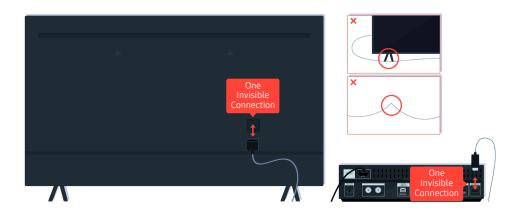
Disconnect and reconnect the One Invisible Connection cable between the TV and the One Connect (OC) Box. Make sure that the One Invisible Connection cable is not pinched or bent sharply.
