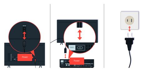
First disconnect and reconnect the power cables and HDMI cables on the back of your TV or the One Connect Box, then unplug the power cable and plug it back into the wall outlet.
