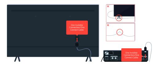
Disconnect and reconnect the One Invisible Connection or One Connect Cable between the TV and the One Connect Box. Make sure that the One Invisible Connection or One Connect Cable is not pinched or bent sharply.
