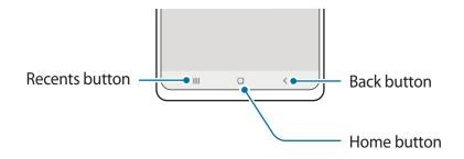
When you turn on the screen, the soft buttons will appear at the bottom of the screen. Refer to Navigation bar (soft buttons) for more information.
