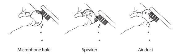
① Do not use anything sharp or excessive force while removing earwax or debris. The microphone hole, speaker, and air duct may be damaged.
