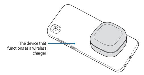
5 After fully charging, disconnect the charging case from the device that functions as a wireless charger.
