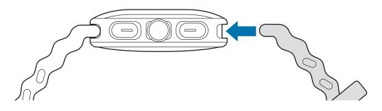
2 Gently pull on both sides of the band to make sure it is tightly connected and not detached from your Watch.
