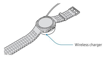
**3** After fully charging, disconnect the Watch from the wireless charger.
