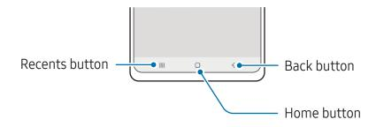
When you turn on the screen, the soft buttons will appear at the bottom of the screen. Refer to Navigation bar (soft buttons) for more information.
