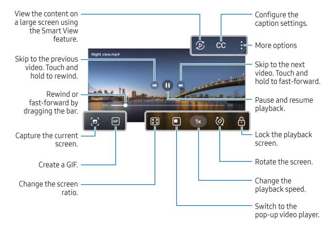
Drag up or down on the left side of the playback screen to adjust the brightness, or drag up or down on the right side of the playback screen to adjust the volume.
