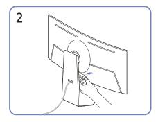
Connect the cables to the corresponding ports.
