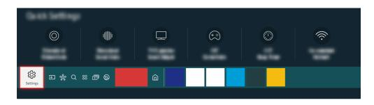
Go to (a) > (b) Settings > Support > Device Care > Self Diagnosis > Sound Test to check the sound.
