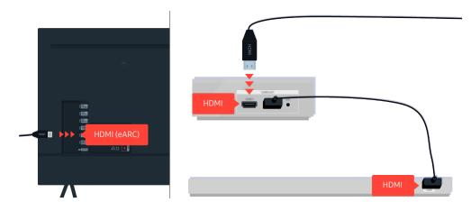
If your Sound Bar is connected to a receiver, and the receiver is connected to the TV using an HDMI cable, check the HDMI connector on the back of the TV. The cable must be connected to the HDMI (eARC) port on your TV.
