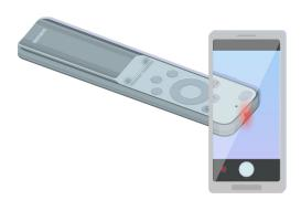
You can check whether the signal is being transmitted by pressing the power button and observing the front tip of the remote control through the camera on your smartphone.
