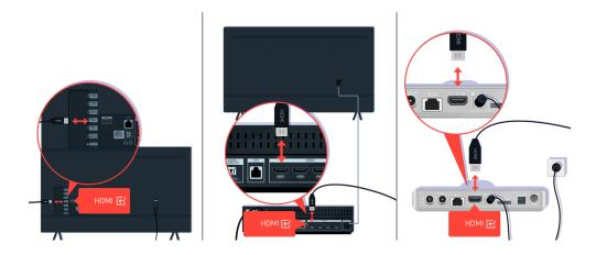
Check the antenna and HDMI cable connections.
