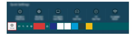
Check the volume on the screen. If a number for the TV volume is not displayed, select > Sound > Sound Output. Then, select TV Speaker.
