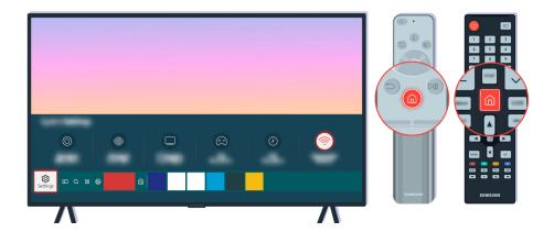
If your TV is connected to the Internet, you can set it to receive periodic updates automatically. On the remote control, press the fall button and move to the Settings using the directional button.
