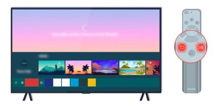
Press the 🕥 and 📵 buttons simultaneously to display the pairing animation clip.
