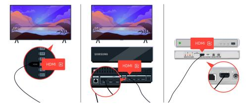
If the same problem continues, try connecting another external device to the TV using an HDMI cable. If the display is correct, your external device may be faulty.
