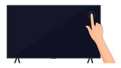
If the TV screen is still blank, softly tap it with your finger. If the part of the screen you tapped on blinks, your TV is correctly connected to the power supply.
