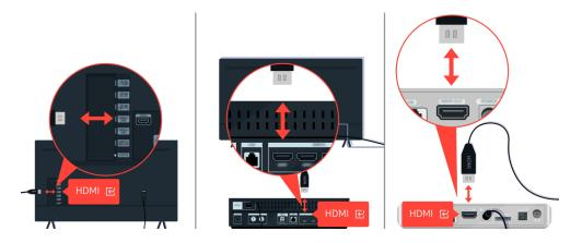
First disconnect and reconnect the power cables and HDMI cables on the back of your TV or the One Connect Box, then unplug the power cable and plug it back into the wall outlet.
