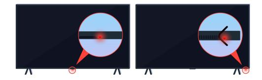
Verify that the infrared remote control signal is being transmitted and received.
