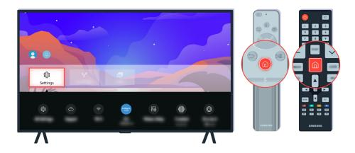
If the same problem persists, run a diagnostic test. On the remote control, press the 🙆 button.
