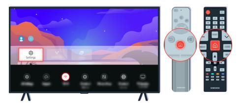
If your TV is connected to the network, you can set it to receive periodic updates automatically. On the remote control, press the final button and move to  $\equiv$  Menu >  $\otimes$  Settings > Support using the directional button.
