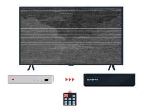
If you use an Multi-Brand Remote (MBR) or universal remote and your remote cannot operate an external device, move the external device closer to the One Connect Box.
